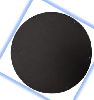
A grid is recommended when x-raying objects that are 10 cm thick or greater. When thick objects are x-rayed they create scattered radiation which contributes to fogging on the image.
