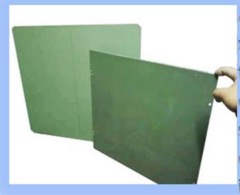
A grid is recommended when x-raying objects that are 10 cm thick or greater. When thick objects are x-rayed they create scattered radiation which contributes to fogging on the image.
